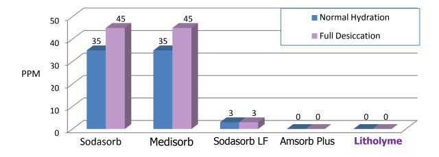
Comparison of Accumulated Carbon Monoxide Production Under Hydrated and Desiccated Conditions
