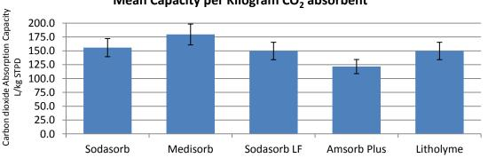
Mean Capacity per Kilogram CO<sub>2</sub> absorbent
